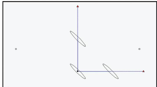
Figure 8: Layout and error ellipses for the free station geometry test observations and positions.
