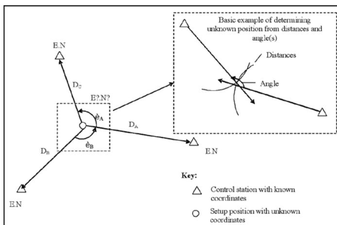
Figure 1: Free station procedure and processes
