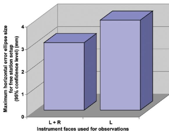
Figure 9: Effect of observing using one or both faces on the horizontal accuracy
