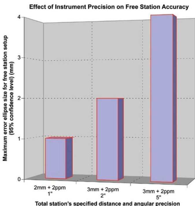
Figure 5: Effect of instrument precision on free station accuracy
