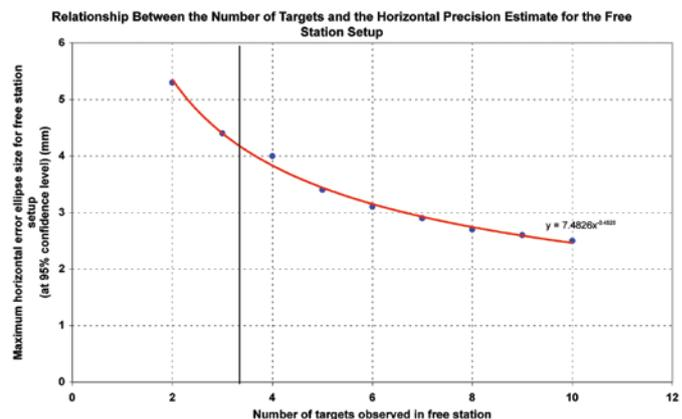
Figure 6: Relationship between the number of targets and the horizontal accuracy estimate for the free station setup
